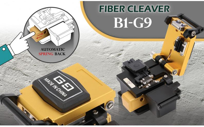
G9 Fiber Cleaver is a high precision optical fiber cleaver is used for precision cutting single core fiber or ribbon fiber. And it not only apply to 250um coated fiber. but also apply to 900um coated fiber, cutting angle is smaller and more precise, easy to use do not need special skills, with automatic spring back function, collaterat collector function.
